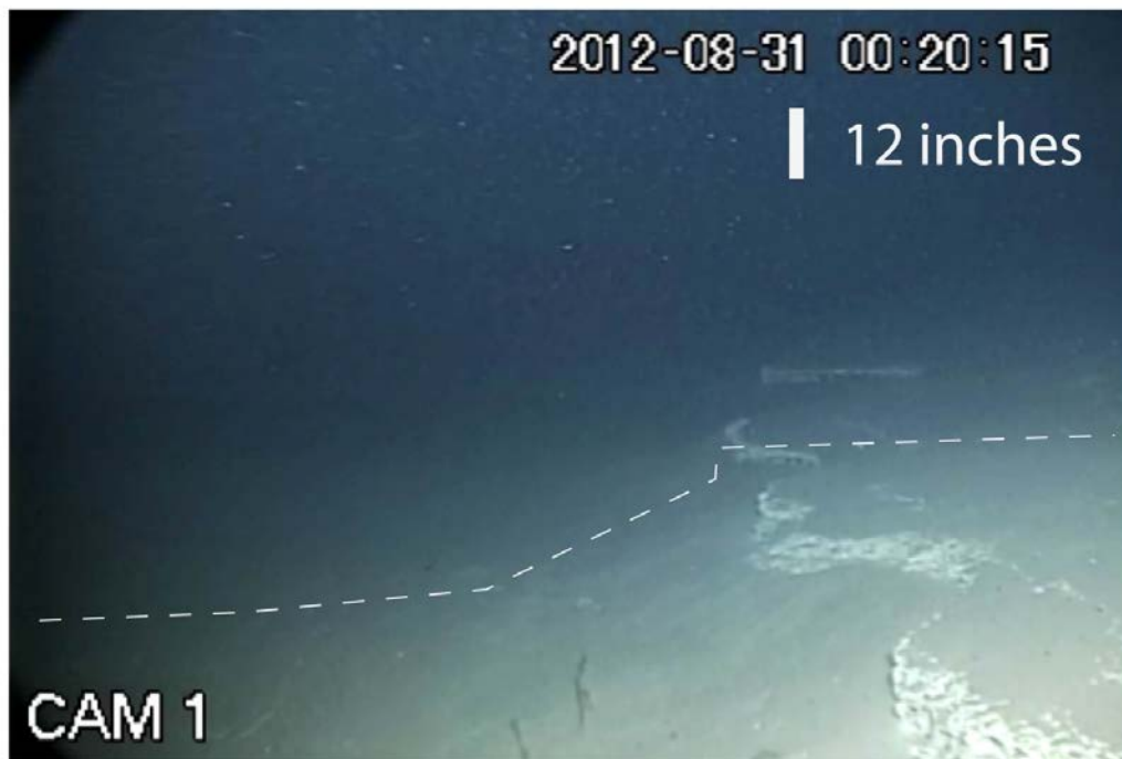
Figure 14. Incipient Landslide West-Facing Head Scarp ROV Image. Site 1. The approximate scale 30 cm (12 inches) applies to the west-facing scarp in the foreground. The dashed line indicates the surface slope profile.
