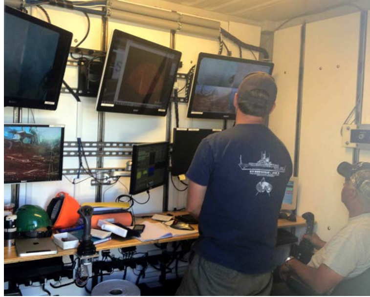
Figure 6. ROV Control Center. Multiple monitors and control joysticks.
