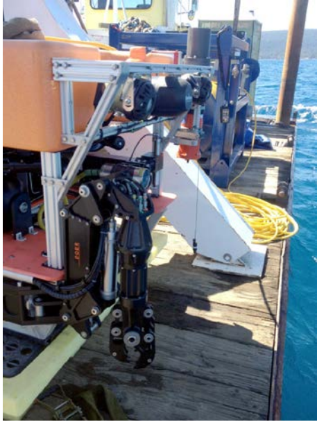
Figure 5. ROV Grab Arm. Camera, lights, yellow tether and winch.
