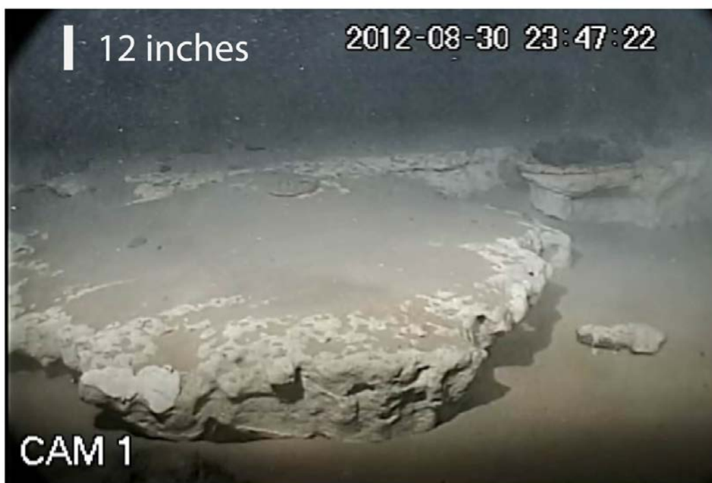
Figure 15. Incipient Landslide East-Facing Head Scarp ROV Image. Site1. The approximate scale 30 cm (12 inches) applies to the scarp in the foreground.
