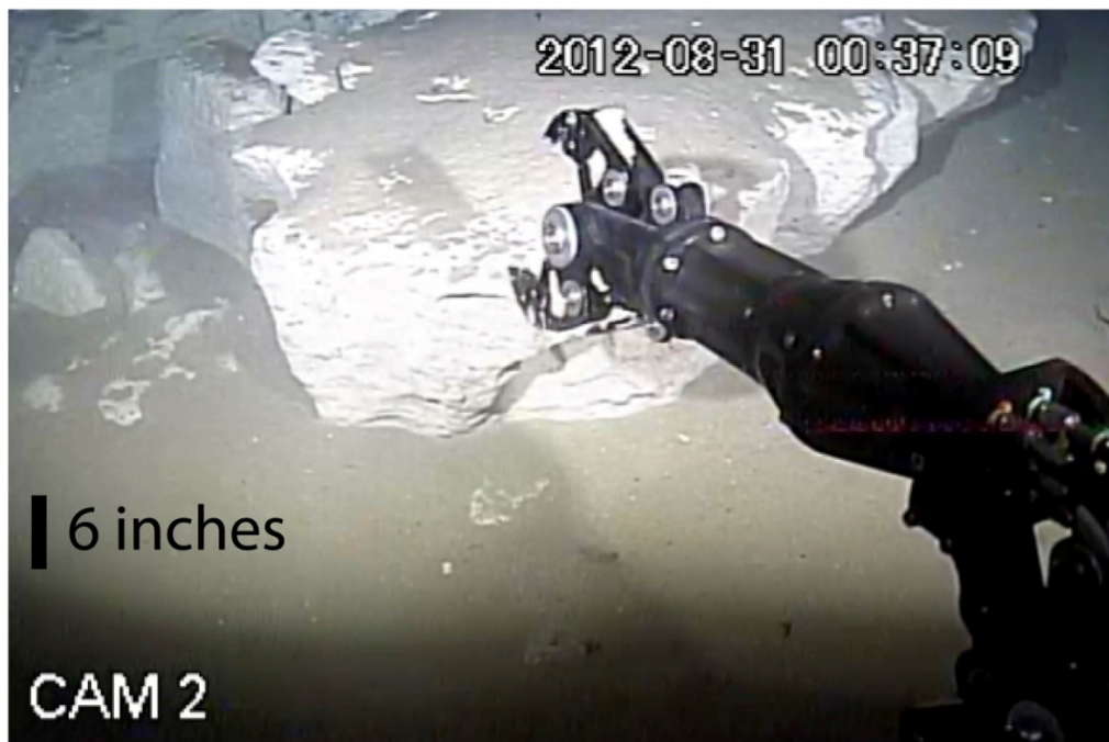
Figure 17. Incipient Landslide East Facing Head Scarp ROV Image. Probing with grab arm. Site 1. The approximate scale 15 cm (6 inches) applies to the scarp in the near field.
