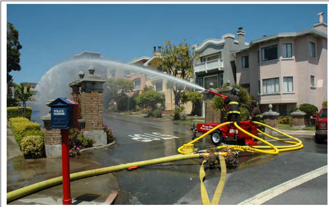
Figure 55 SFFD portable monitor deploying a water curtain (source: http://sfearthquakesafety.org/the-bond/firefighting-water-supply-system/ ).
