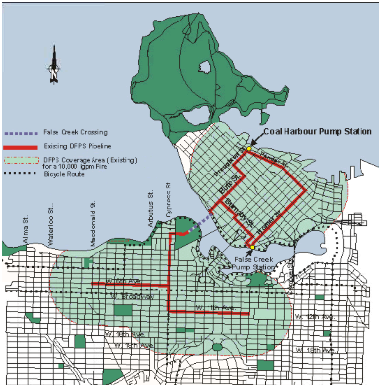
Figure 39 Plan of Vancouver, B.C. Dedicated Fire Protection System.
