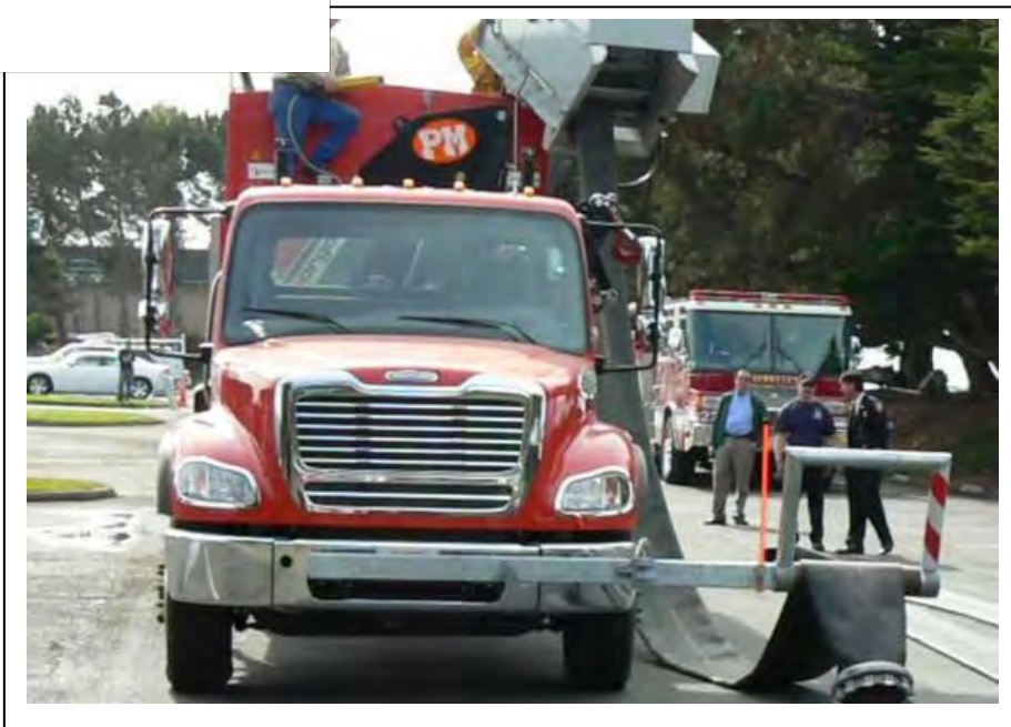
Figure 44 Berkeley FD BAWSS – (top) HydroSub unit, (mid) 12 inch Ultra LDH being flaked out from transporter-borne container, and (bottom) hose being reeled back into container.
