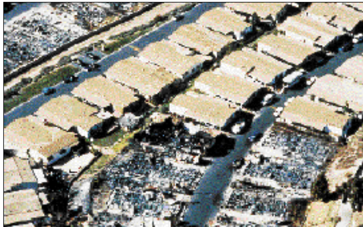
Figure 47. One hundred seventy-two mobile homes burned in this earthquake. Fires most often started because of severed gas lines.
